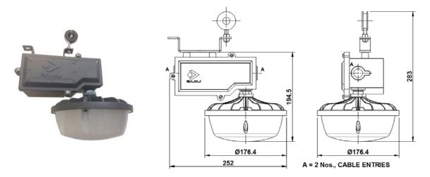
Dimensions in mm Tolerance +/-5mm
