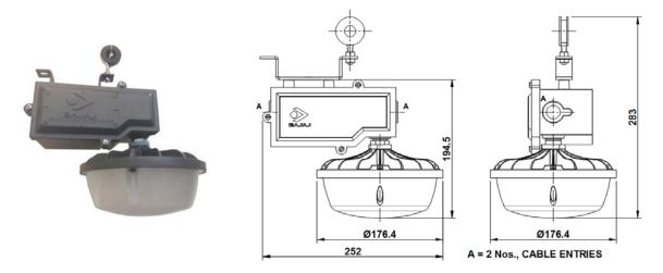
Dimensions in mm Tolerance +/-5mm
