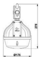
Dimensions in mm Tolerance +/-5
