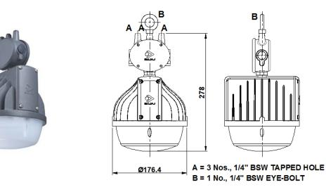
Dimensions in mm Tolerance +/-5mm
