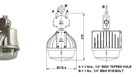
Dimensions in mm Tolerance +/-5mm
