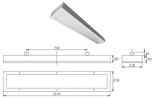
Dimensions in mm Tolerance = +/-5
