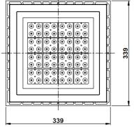
NOMINAL DIMENSIONS IN mm Tolerance +/-5mm
