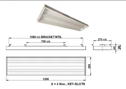
Dimensions in mm Tolerance: +/-5
