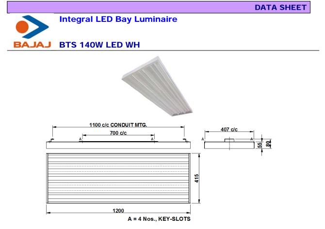
Dimensions in mm Tolerance: +/-5
