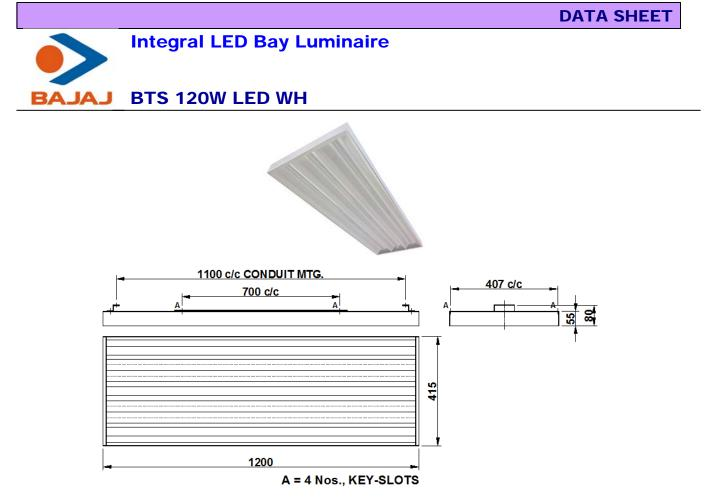
Dimensions in mm Tolerance: +/-5
