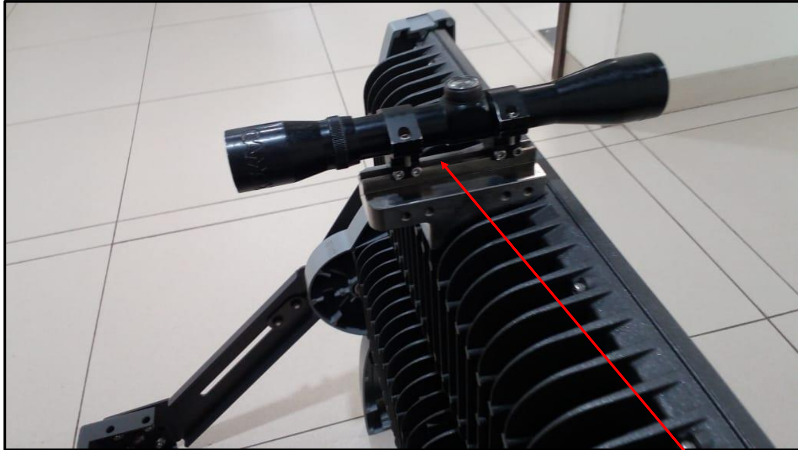
Precise slot to fix the 'aiming device'
